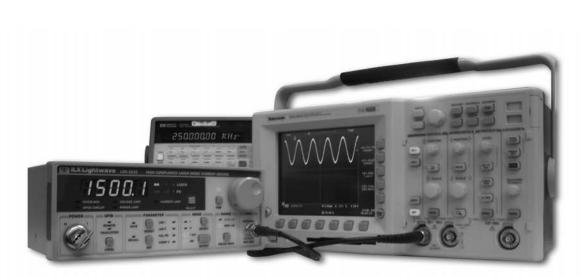
LDX-3200 Series Current Sources can be analog modulated with an external input to 1MHz.
